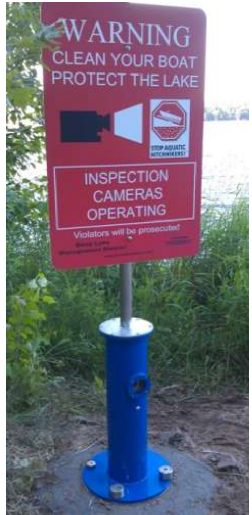
Photo shows I-LID in position at the boat-launching site with warning sign to "Clean Your Boat". Note camera aperture on side of vertical mounting tube.
